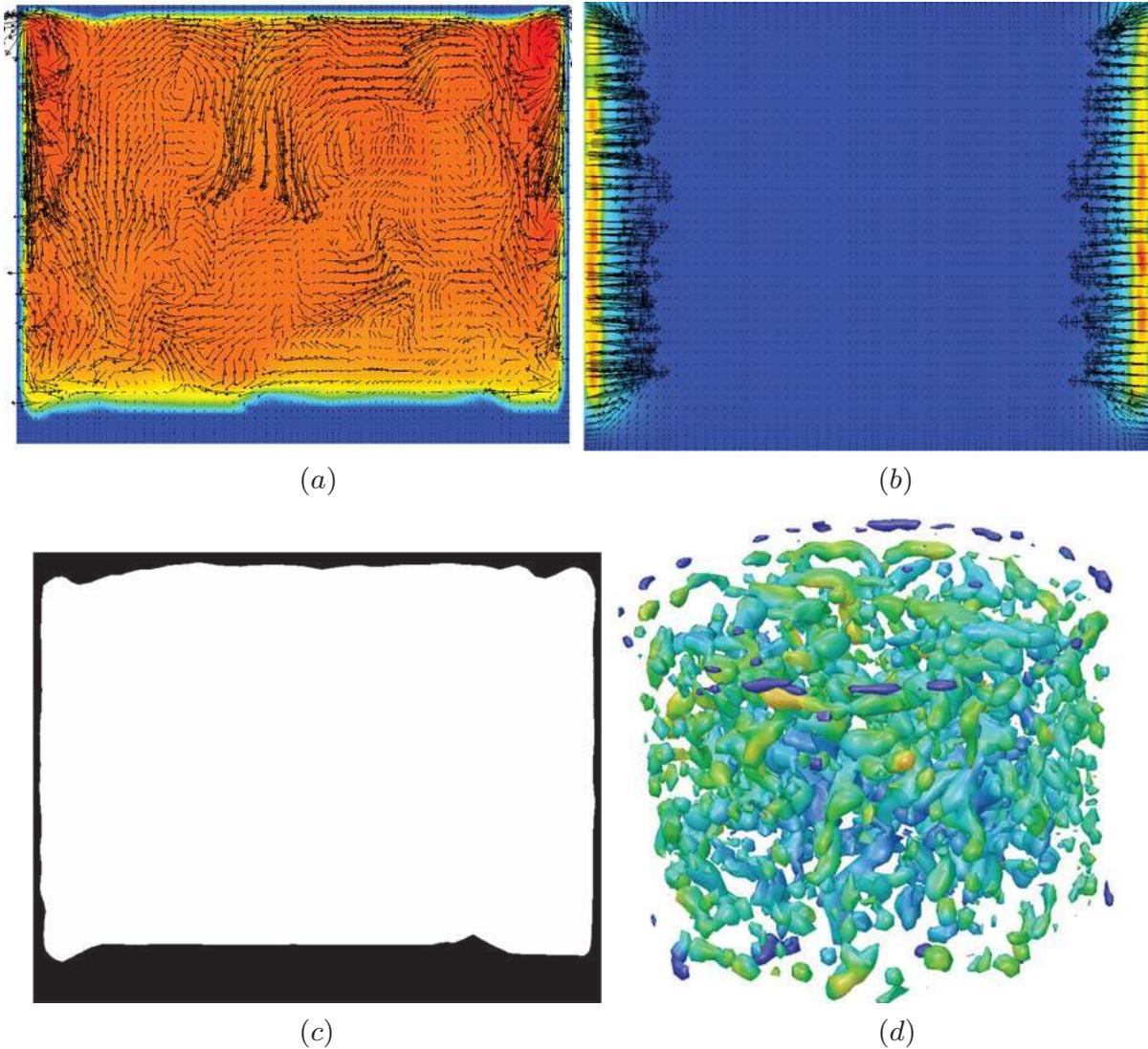
Fig. 3. Some typical results obtained after global thermal stabilization. (a) Temperature (range 2800–3277 K) and velocity vectors ( $V_{\max} = 0.03$  m/s). (b) Joule power (Max:  $7662 \text{ Wm}^{-3}$ ) and Lorentz forces vectors (Max:  $6400 \text{ Nm}^{-3}$ ). (c) Crust profile defined by viscosity (black: solid, white: liquid). (d) Iso-contours of  $Q$ -criterion.
