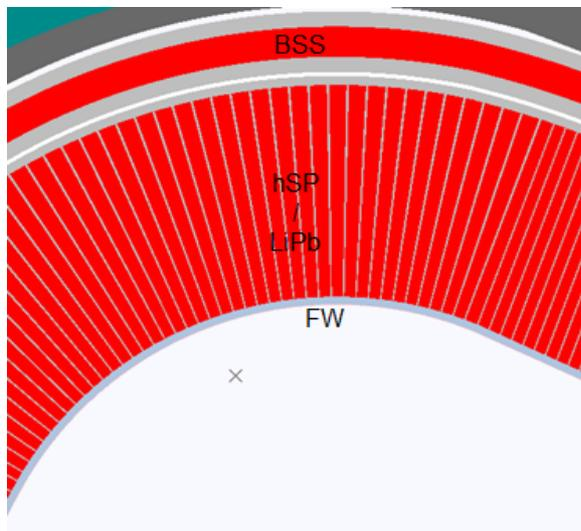
Fig. 2 Radial – poloidal cut of the upper part of inboard segment (color legend: LiPb – red, eurofer – gray, VV 1<sup>st</sup> layer – deepgray, VV 2<sup>nd</sup> layer – darkcyan). (For interpretation of the references to colour in this figure legend, the reader is referred to the web version of this article.)
