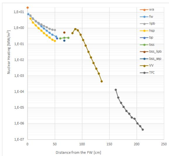
Fig. 6 NH density radial profile at inboard
