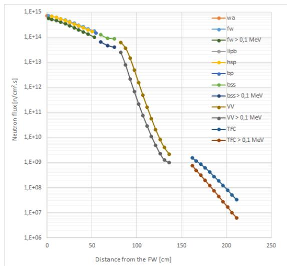
Fig. 5 neutron flux radial profile at inboard
