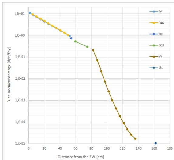
Fig. 7 displacement damage radial profile at inboard
