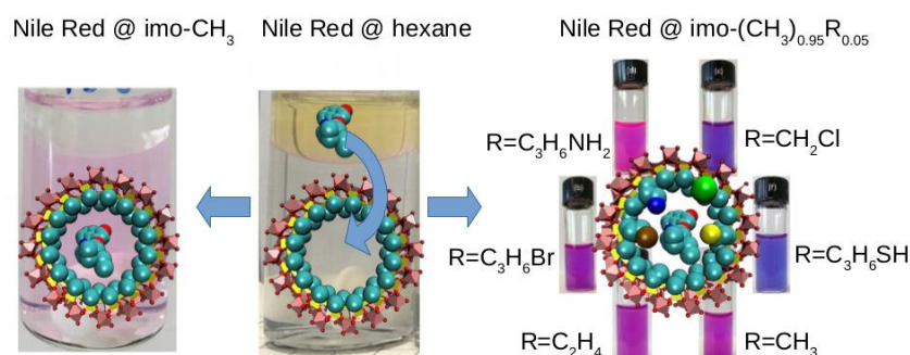
Figure 1 : Liquid liquid extraction of Nile Red and impact of internal surface doping with Si-R groups on the optical properties of encapsulated molecules.
