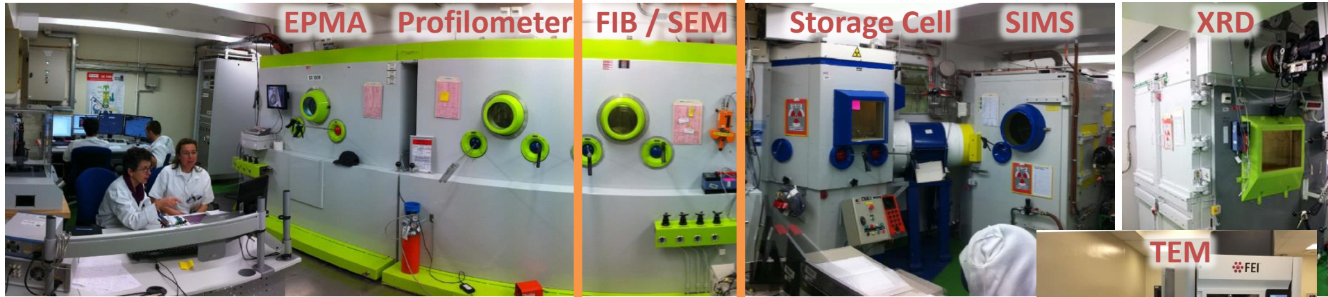
The front shielded wall
