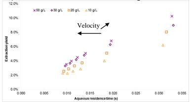
Figure 1. Uranium(VI) extraction yields versus aqueous residence, function of the initial uranium(VI) concentration.
