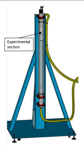
Fig. 5. View of designed experimental test section located on the supporting frame
