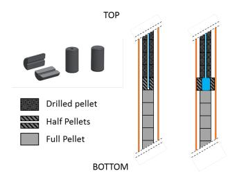
Fig. 3. Schematic view of the functioning of expansion system to induce pellet-clad interaction: inflation of the balloon through the shaft leads to fake-pellets displacement inducing pellet-clad contact in a localized region of the sample rod.
