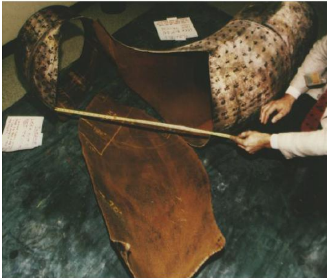
Surry 2: blow up of a 18" elbow
