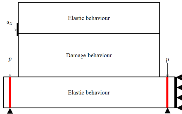
Fig. 15 Principle of the experimental device for the loading and the boundary conditions
