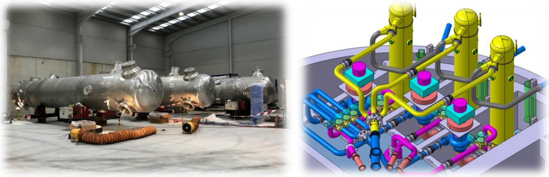
Fig. 5: Primary heat exchangers in factory
