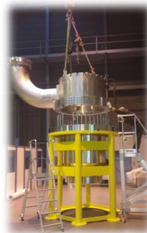
Fig. 4: Core block assembly in factory
