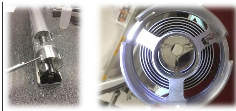
Fig. 7: Dimensional controls of a dummy fuel assembly
