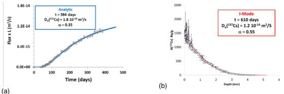
Figure 2: Cs-137 diffusive flux (\*L) in the Na<sub>2</sub>SO<sub>4</sub> SUB-MIX1 system (a) and Cs-137 diffusive profile in the NaNO<sub>3</sub> CEA-MIX1 system (b). Solid lines represent Subatech (blue) and CEA (red) best fit modeling curves.
