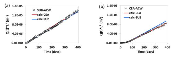
Figure 1: Comparison of HTO normalized total activity experimental data and modeling as a function of time (up to 400 days) in ACW. Experimental data from Subatech and CEA are plotted in Fig 1 (a and b) respectively. Solid lines represent Subatech (blue) and CEA (red) best fit modeling curves.
