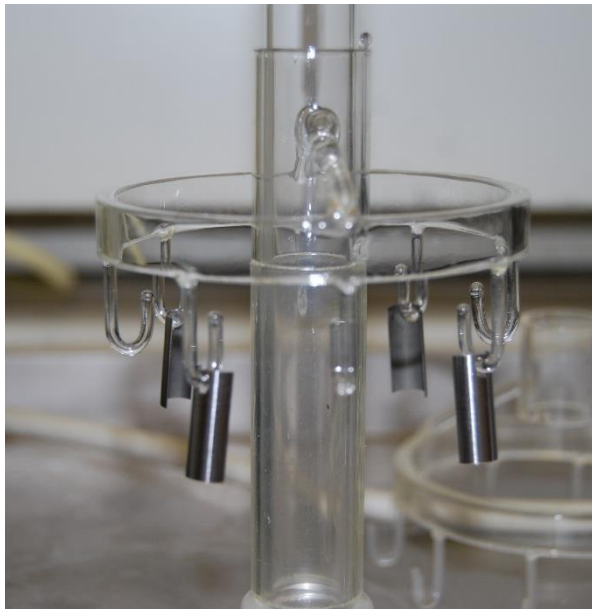
4 corrosion coupons hung up on a circular sample holder
