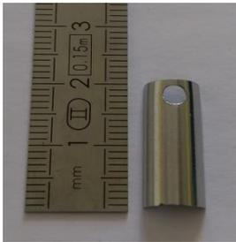
Tile-shaped corrosion coupons
