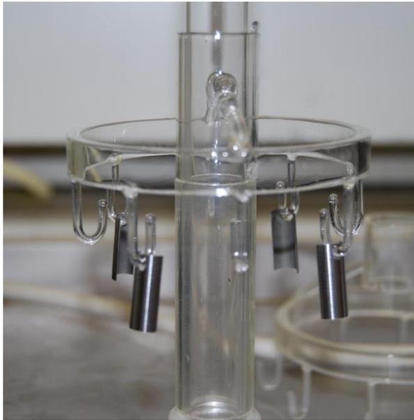
*Corrosion coupons hung up on a circular sample holder*
