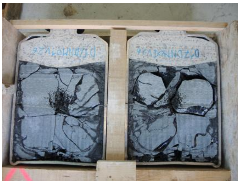
Fig. 3. Canister of the IN CAN MELTER cut in half after vitrification preliminary tests of a dismantling tank deposit high level waste.
