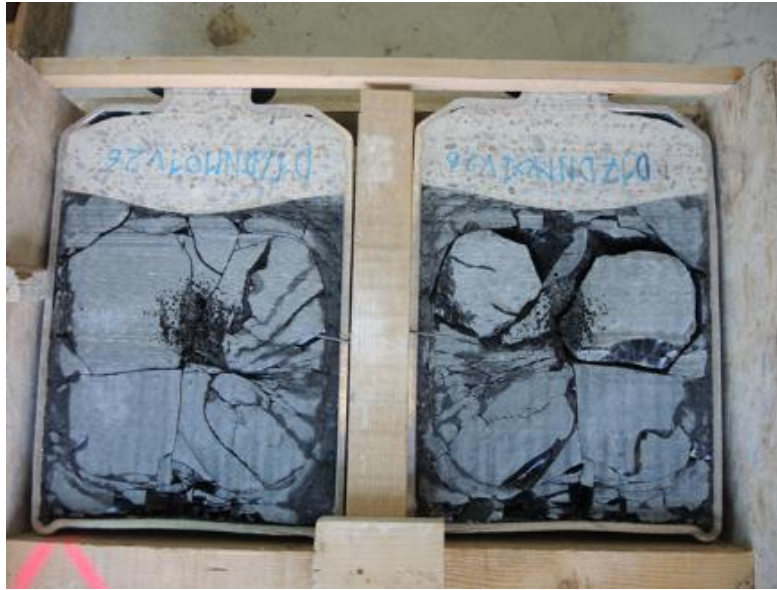
Fig. 3. Canister of the IN CAN MELTER cut in half after vitrification preliminary tests of a dismantling tank deposit high level waste.
