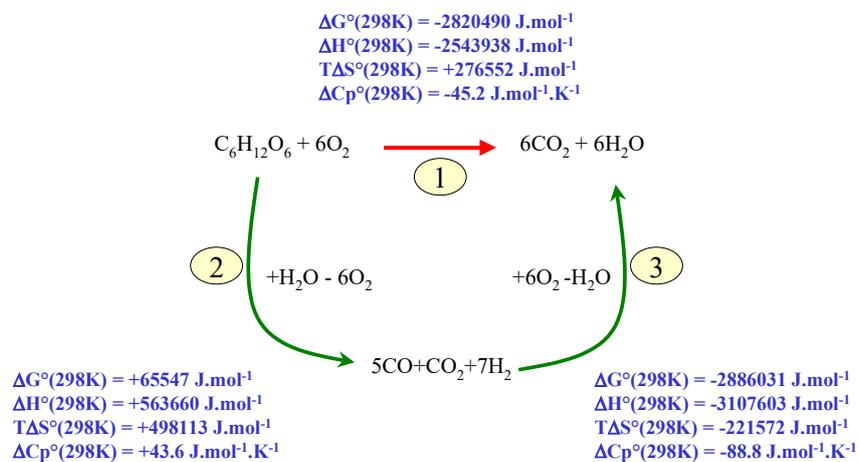
Figure 10: Two paths for heat production from cellulose.
