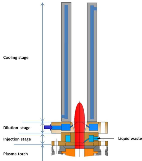
**Figure 4:** Schematic view of the combustion zone.
