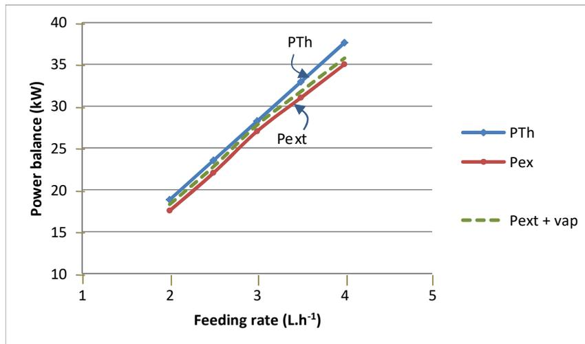
**Figure 7:** Comparison between theoretical power dissipated during treatment with variable TBP-Dodecane feeding rate and the measured power.
