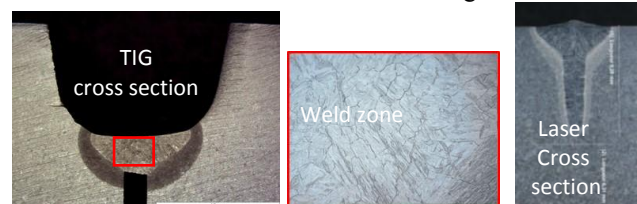
Figure 3: cross sections of TIG and laser welds
