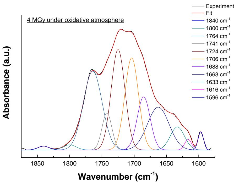
ATR mode infrared spectra with subtraction of the pristine PS spectrum
