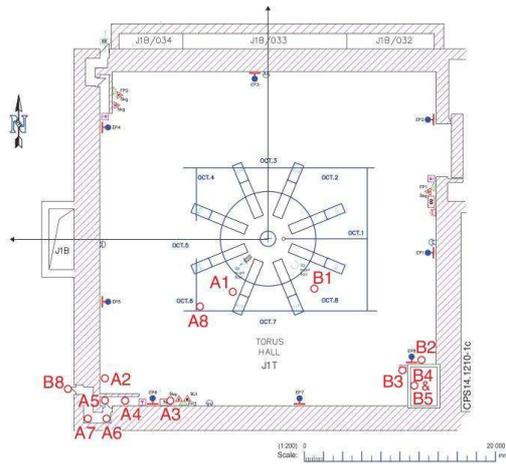
Fig. 1 JET Torus Hall (Dosimeters locations A1-A8 and B1-B8) (see Reference [2])
