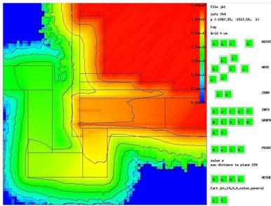
Fig. 6. TRIPOLI-4 calculated ambient dose equivalent map for neutrons and iso-dose rates curves around the JET-like maze entrance. (X-Y cross sectional view).
