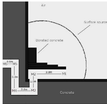
Fig. 2 Cross sectional view of the SW entrance maze of JET [2-3]
