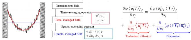
Optional terms can be added in momentum and energy balance equations to model turbulent diffusion and dispersion effects. These terms have an impact on core simulation at subchannel scale. So, the CATHARE team had established models for these terms in rod bundle geometry and had validated them on various rod bundle experiments [2].
