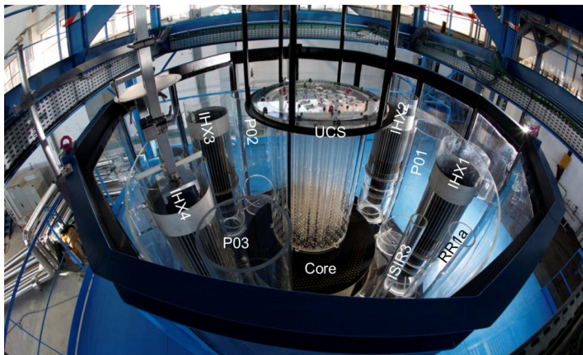
Fig.2. Top view of the MICAS mock-up (P0x stands for the pump pit, UCS, for the Upper core Structure, IHXx, for the Intermediate Heat Exchanger, ISIRx, for the inspection in operation, RRxa, for the decay heat exchanger)
