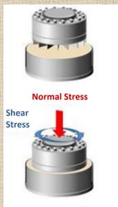
FT4 Powder Rheometer Shear cell [4]
