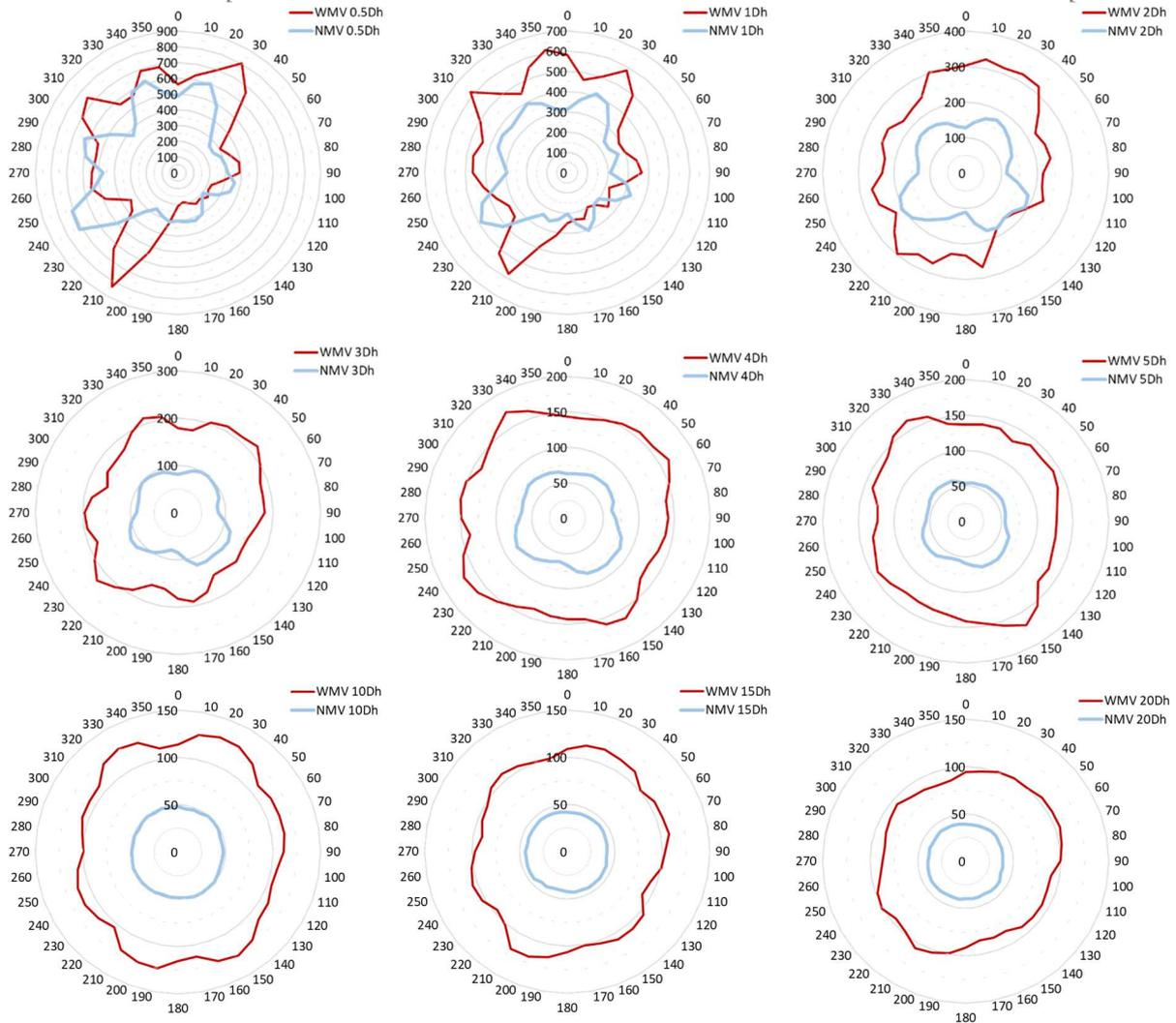
Fig. 3 azimuthal distributions of the rms of the pressure fluctuations  $P'_{rms}$  [in Pa] for the cases of grids with mixing vanes (WMV) and without mixing vanes (NMV) for different vertical distances from the grids, i.e.  $0.5D_h$ ,  $1D_h$ ,  $2D_h$ ,  $3D_h$ ,  $4D_h$ ,  $5D_h$ ,  $10D_h$ ,  $15D_h$  and  $20D_h$ .
