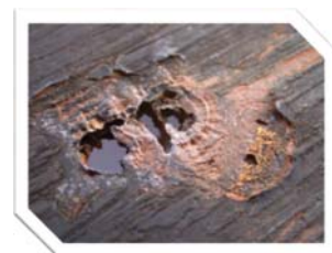
Pitting corrosion of an oil tank
