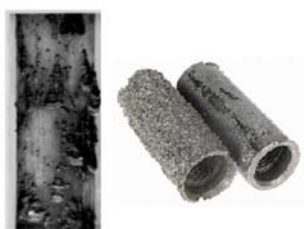
Corrosion of pipes in SCCO 2 storage system from G. Schmitt, White paper, WCO, 2009
