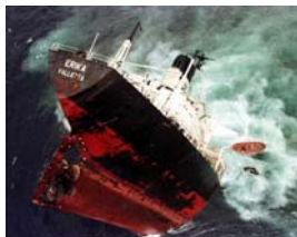
ERIKA (1999) "result of structural weakness caused by corrosion"
