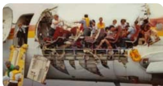
Corrosion cracking of the fuselage of airplane (April 28, 1988 – 1 fatal over 95)
