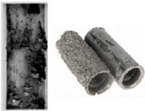
Corrosion of pipes in SCCO 2 storage system from G. Schmitt, White paper, WCO, 2009
