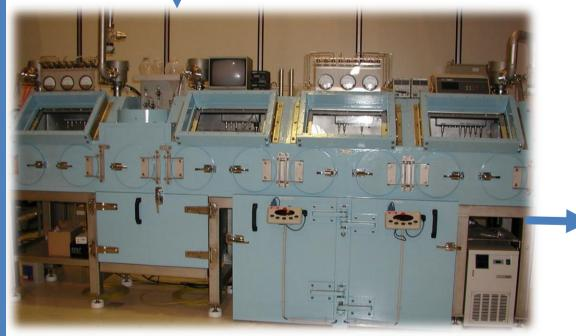
Shielded glove box for the electropolishing machine
