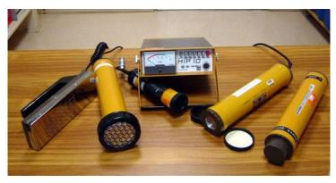
Typical surface contamination detector
