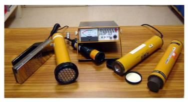
Typical surface contamination detector
