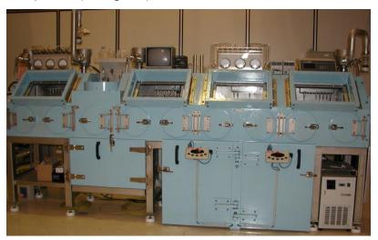
Figure 4. The glove box for the electopolishing machine
