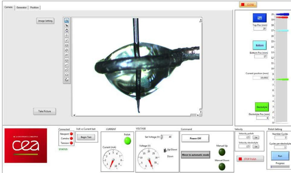
**Figure 5.** Print screen of the interface of the electropolishing machine software developed by CEA
