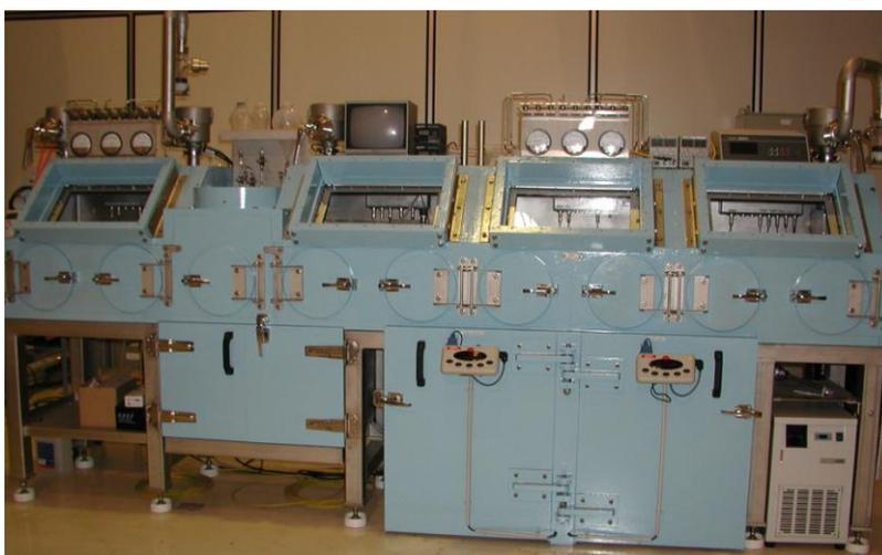
**Figure 4.** The glove box for the electropolishing machine
