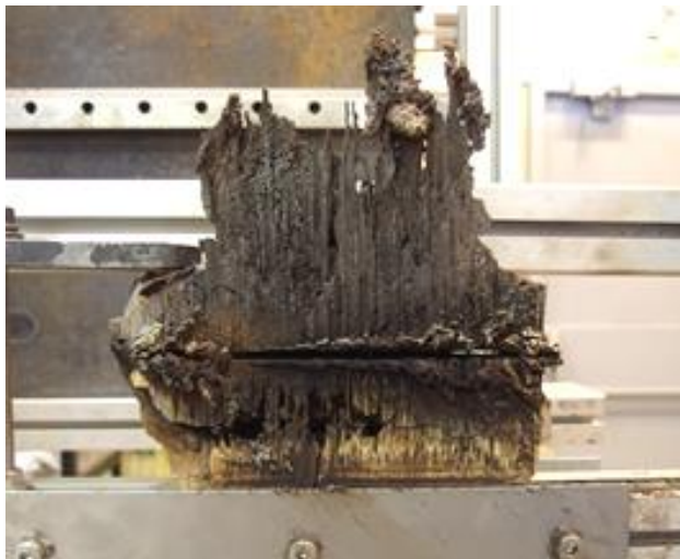
Figure 4. View of laser-cut fuel debris simulant for in-vessel configuration
