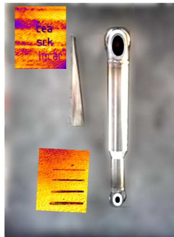
Figure 30: In sodium imaging of a plate with slits and letters (VENUS tests with TUSHT transducers). Optical image (top left), rough acoustic echoes (top right, in blue) and enhanced signal treatment (bottom, orange zones).
