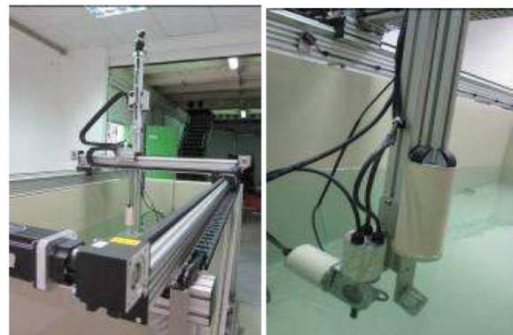
Figure 24: VISIO water facility (2 m long, 1 m large, 1 m height) devoted to ultrasonic visualization study
