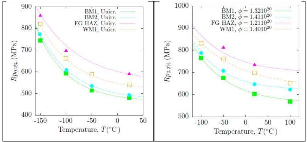
Figure 2: Yield stress (Rp0.2) evolution with temperature for base metals (BM1 and BM2), weld metal (WM1) and fine grain HAZ.
