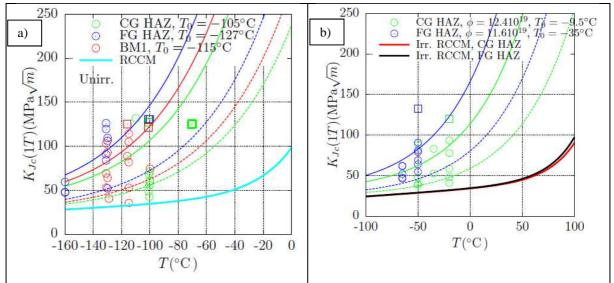
Figure 4: Fracture toughness (1T) for UHAZ (CH HAZ and FG HAZ) as a function of temperature. a: Unirradiated state, b: irradiated. Solid and dotted lines represent the 50% and 2% fractile of master-curve, respectively. Square symbols correspond to censored data with  $K_{Jc} > K_{Jc}$ (limit).
