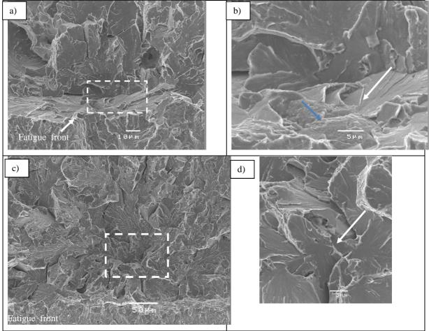
Figure 7: Fractographic investigations of BM1 at the irradiated state. a) and b): KJc (1T) = 31 MPa.m<sup>0.5</sup> at -50°C, c) and d): KJc (1T) = 83 MPa.m<sup>0.5</sup> at -20°C. White arrows indicate the initiation site of cleavage fracture. Blue arrow on b) indicates a decohesion facet.
