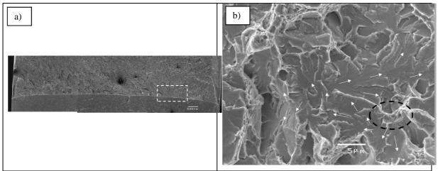
Figure 10: Fractographic investigations of FG-HAZ. Irradiated specimen: KJc (1T) = 54.8 MPa.m<sup>0.5</sup> à-50°C. a) location of the initiation area on the fracture surface. b) Initiation site of cleavage fracture (indicated by a dashed line)
