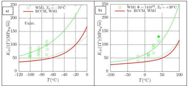
Figure 6: Fracture toughness (1T) for WM1 as a function of temperature. Left: Unirradiated state, Right: irradiated. Solid and dotted lines represent the 50% and 2% fractile of master-curve, respectively. Solid symbols correspond to censored data with  $K_{Jc} > K_{Jc}$ (limit). Initial RT<sub>NDT</sub> value is -48°C
