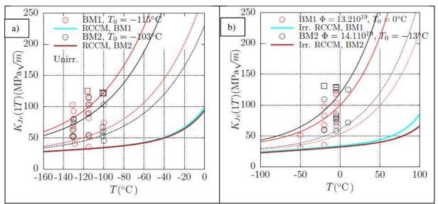
Figure 3: Fracture toughness (1T) for base metals (BM1 and BM2) as a function of temperature. a: Un-irradiated state, b: Irradiated. Full and dotted lines represent the 50% and 2% fractile of master-curve, respectively. Square symbols correspond to censored data with  $K_{Jc} > K_{Jc}$ (limit). Initial  $RT_{NDT}$  values are -27°C and -25°C for BM1 and BM2, respectively.
