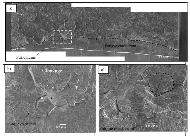
Figure 9: Fractographic investigations of CG-HAZ. Irradiated specimen :  $KJc (1T) = 48.1 MPa.m^{0.5} à-20^{\circ}C. a)$  location of the initiation area on the fracture surface. b) Intergranular facets (IG) at the initiation site. c) coarse facet indicated by dashed line.
