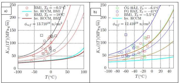
Figure 5: Comparison of fracture toughness (1T) after fluence and temperature normalization. a: Base metal at 13.7  $10^{19}$  n/cm<sup>2</sup>, b: CH HAZ and FG HAZ and base metal at 12.4  $10^{19}$  n/cm<sup>2</sup>. Solid and dotted lines represent the 50% and 2% fractile of master-curve, respectively. Square symbols correspond to censored data with K<sub>Jc</sub> > K<sub>Jc</sub>(limit).
