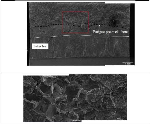
Figure 8: Fractographic investigations of CG\_HAZ at unirradiated state. KJc (1T) = 36.5 MPa.m<sup>0.5</sup> à-115°C. Top: location of the initiation area on the fracture surface. Bottom: mixed mode of transgranular cleavage fracture and
