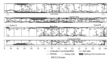
Figure 3: Crack patterns due to corrosion [17]
