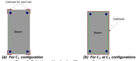
Figure 9: Cathode position for the different configurations
