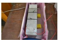
(a)  $C_1$  configuration (b)  $C_2$  configuration (c)  $C_3$  configuration Figure 7: Accelerated corrosion performed on small-scale specimens
