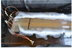
Figure 10 :  $C_1$  beam configuration subjected to accelerated corrosion
