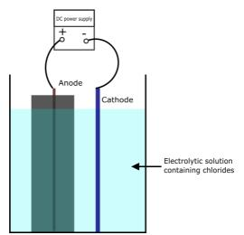
Figure 1: Set-up for accelerated corrosion by imposed current
