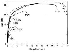
Figure 2: Evolution of corroded steel bars ductility [16]
