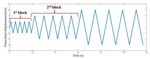
Figure 12: Planned load in quasi-static testing
