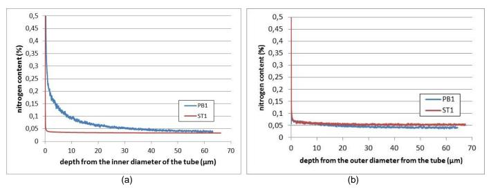
Figure 4: Nitrogen profiles obtained from the inner (a) and outer (b) diameters for PB1 and ST1 respectively
