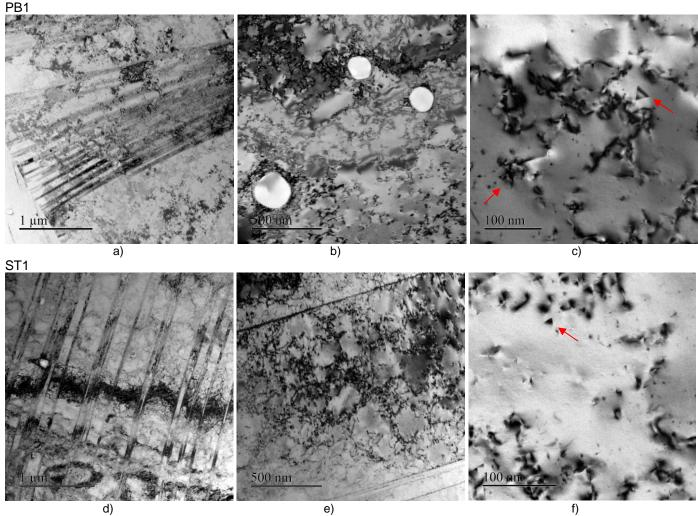
Figure 5: Bright-field TEM micrographs showing the general microstructure with twins, high dislocation density and few dislocation cells as well as TiMoC precipitates and triangular-shaped defects (right images) indicated by the red arrows
