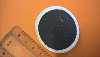
Figure 6 : Photographs of a sample before and after selective dissolution and the collected residue on a nitrocellulose filter with a pore size of 220 nanometers
