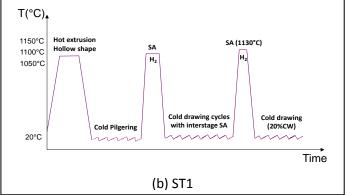
Figure 1: Diagram of fabrication process a) for PB1 and b) for ST1
