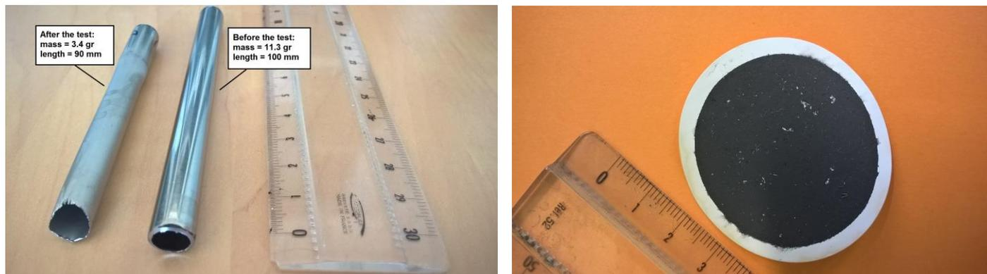
**Figure 6 : Photographs of a sample before and after selective dissolution and the collected residue on a nitrocellulose filter with a pore size of 220 nanometers**
