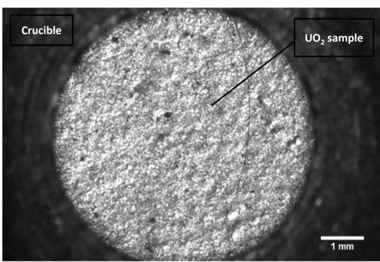
*Observation of a UO<sub>2</sub> pellet* with the optical system
