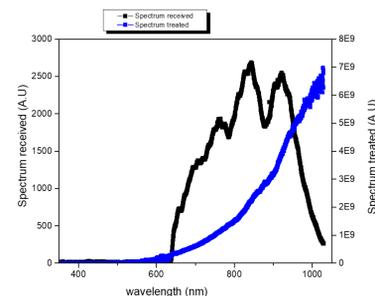
Spectrum as received from the spectrometer of a UO<sub>2</sub> pellet heated at 1200°C (black) and after processing with the inverse transfer function (blue)
