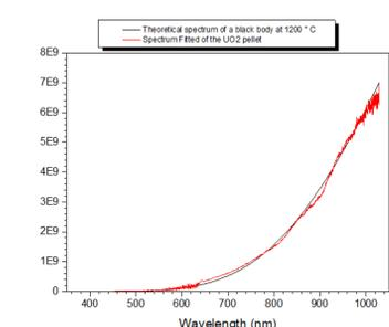
Measured spectrum of a heated UO<sub>2</sub> pellet (red) and fitted with Planck's law at 1200°C (black)
