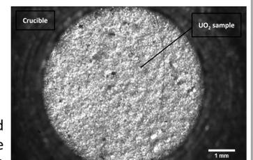
Observation of a UO<sub>2</sub> pellet with the optical system
