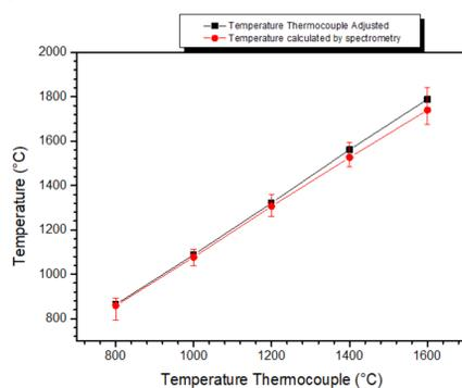
Temperature of the sample from the qualification phase and, as determined, by multispectral pyrometry
