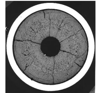
PHENIX pellet, initially solid Final burn-up : 13,3 at%
