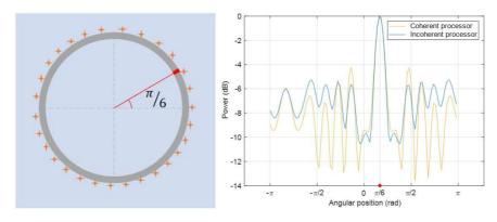
Figure \*: Detection of a local defect with Matched Field Processing
