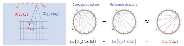
Figure \*: Match Field Process principle (left). Measured and forward acoustic fields. Subtracting operation between reference and damage states (right)
