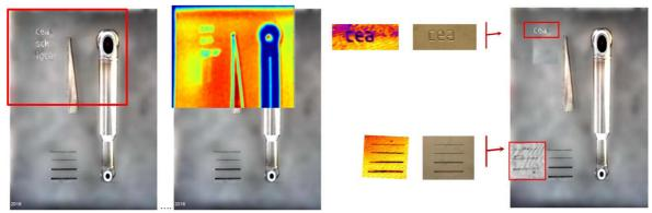
Figure \*: Ultrasound images of the VISION mock-up: triangle, pipe, grooves and letters, with flat front face TUSHT Ø40 mm coupled with focusing lens (at 6.5 ± 0.4 MHz)
