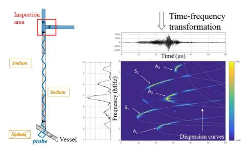
Figure \*\*: Inspection configuration (left) and modal identification (right)
