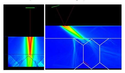
Figure \*\*: Examples of beam visualization in the weld from ATHENA2D calculation for L0 wave (left) and SW45 (right)
