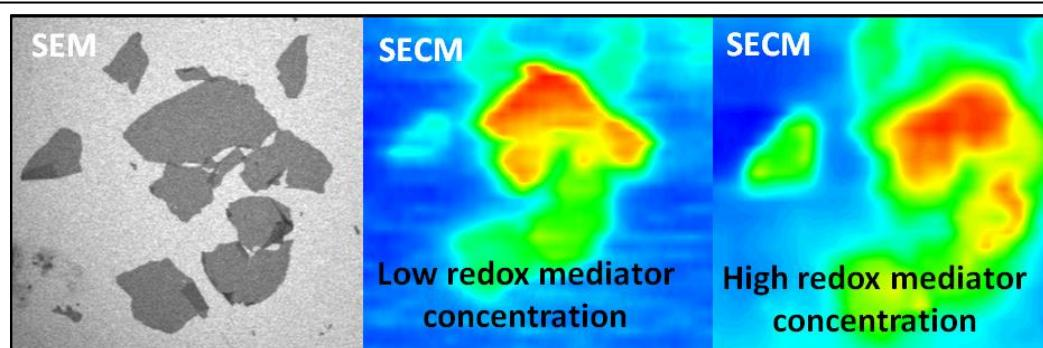
**Fig. 1:** Presentation of the combined SEM-SECM responses at the basis of an advanced electronic transport characterization. Taken from 3
