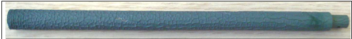
Fig 5. Typical PQ aspect of a Cr-coated M5 after HT oxidation at 1400°C
