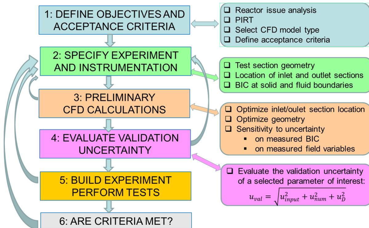
Figure 3: Roadmap for designing and performing a CFD-grade experiment
