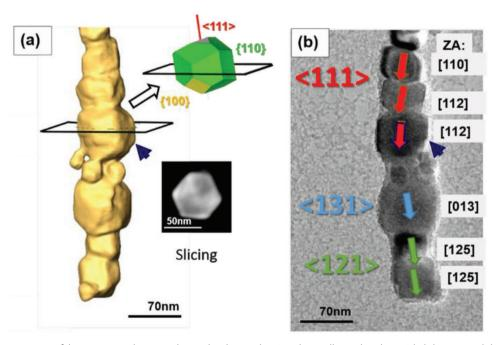
Figure 3. a) ET reconstruction of the magnetite chain (synthesized without gelatin) and crystallographic shape (slightly truncated rhombidodecahedra) for one selected NC and b) respective HRTEM image illustrating the crystallographic orientation of magnetite NCs.
