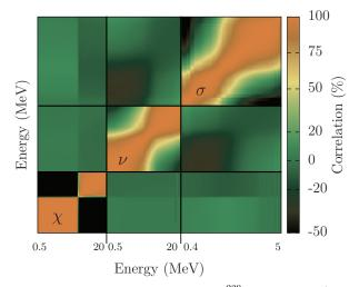
**Fig. 5.** Posterior correlation matrix for  $^{239} Pu \ \nu, \sigma$  and  $\chi$  (for the incident neutron energy of 750 keV). The energy axis is for the incident neutrons for  $\nu$  and  $\sigma,$  and for the outgoing neutron for  $\chi.$  The X- and Y-axis are in linear scale.
