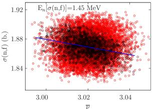
Fig. 1. Example of correlations between  $\nu$  and  $\sigma$  for two different incident neutron energies for the fission cross section. The incident neutron energy for  $\nu$  is 900 keV in both cases. The considered criticality benchmark is pmf1. 10 000 samples are presented; the distinct colors are proportional to  $w_i$ : red for small  $w_i$  and black for  $w_i \simeq 1$ .
