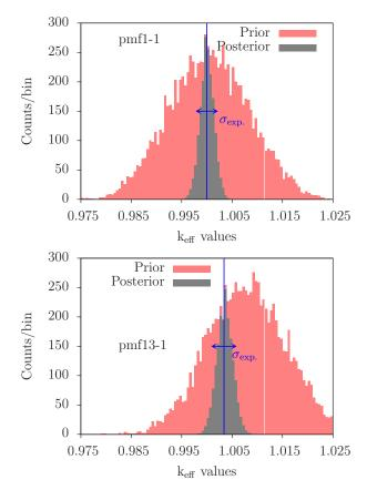
Fig. 4. Prior and posterior distributions of  $k_{\rm eff}$  for two benchmarks: pmf1 and pmf13. The blue line indicate the experimental value with its uncertainty.
