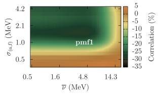
**Fig. 3.** Correlation matrix between  $^{239}$ Pu  $\nu$  and  $\sigma$  considering the fast pmf1 benchmark. The X- and Y-axis are in log scale.
