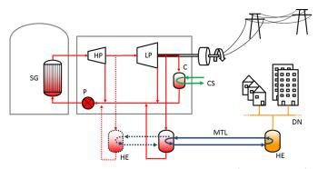
Fig. 2. Diagram of nuclear cogeneration for DH (personal work).
