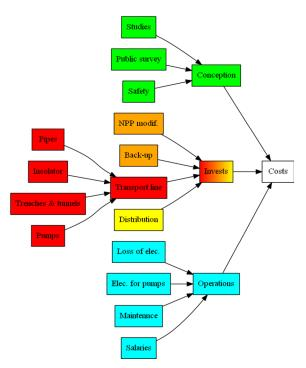
Fig. 3. Cost breakdown structure.
