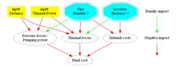
Fig. 4. Simplified chart of the main interactions between the critical variables of the system.
