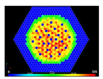
**Fig. 2.** Linear power distribution (W/cm by pin) in the center of the core at beginning of cycle.
