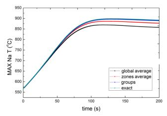
Fig. 8. Sodium maximal temperature during ULOF/PP accident for different thermal properties models.
