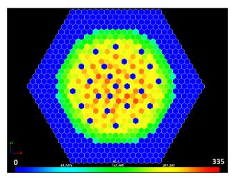
**Fig. 3.** Linear power distribution (W/cm by pin) in the center of the core at end of cycle.
