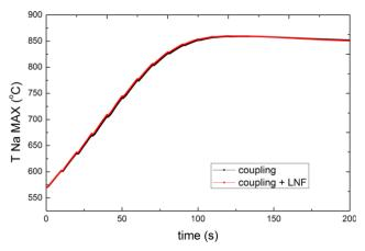
Fig. 19. Sodium maximal temperature during ULOF/PP accident with coupling and different Doppler effect treatments.
