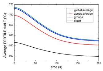
Fig. 11. Average fertile temperature during ULOF/PP for different  $H_{qap}$  treatments.
