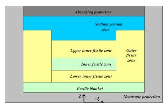
Fig. 1. Scheme of the CFV core concept.
