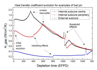
Fig. 4. Typical heat transfer coefficient evolution for chosen sub-assemblies (in top fissile zone).
