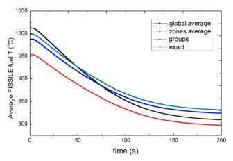
Fig. 10. Average fissile temperature during ULOF/PP for different  $H_{gap}$  treatments.
