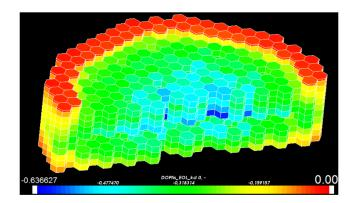
Fig. 12. 3D map of Doppler coefficients (pcm) in fissile zones.
