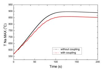
Fig. 15. Sodium maximal temperature during ULOF/PP accident with and without coupling.
