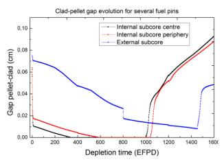
**Fig. 5.** Typical gap size evolution for chosen sub-assemblies (in top fissile zone).
