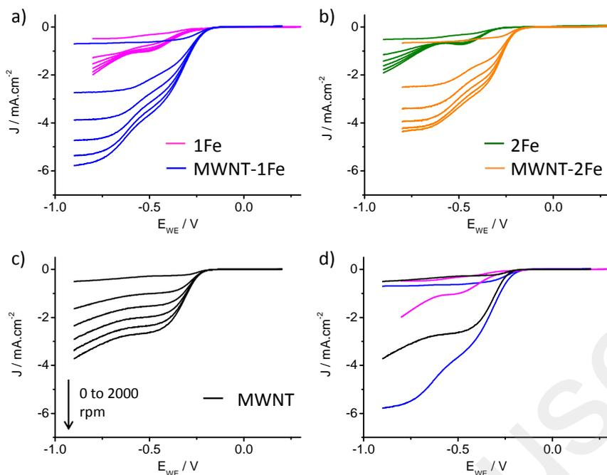
**Figure 3.** Polarization curves at different rotation rates (0, 400, 800, 1200, 1600 and 2000 rpm) recorded for ORR in  $O_2$ -saturated 0.1 M NaOH solution (pH 13) (scan rate = 5 mV/s, room temperature) on GC with predeposited (a) **1Fe** (pink) and **MWNT-1Fe** (blue); (b) **2Fe** (green) and (c) **MWNT-2Fe** (orange); **MWNT** (black). (d) Comparison between **MWNT**, **MWNT-1Fe** and **1Fe** at 0 and 2000 rpm.
