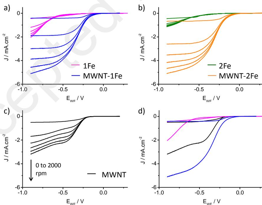
**Figure 4.** Polarization curves at different rotation rates (0, 400, 800, 1200, 1600 and 2000 rpm) recorded for ORR in  $O_2$ -saturated at pH 10 (phosphate buffer solution) (scan rate = 5 mV/s, room temperature) on GC with predeposited (a) **1Fe** (pink) and **MWNT-1Fe** (blue); (b) **2Fe** (green) and **MWNT-2Fe** (orange); (c) **MWNT** (black). (d) Comparison between **MWNT**, **MWNT-1Fe** and **1Fe** at 0 and 2000 rpm.
