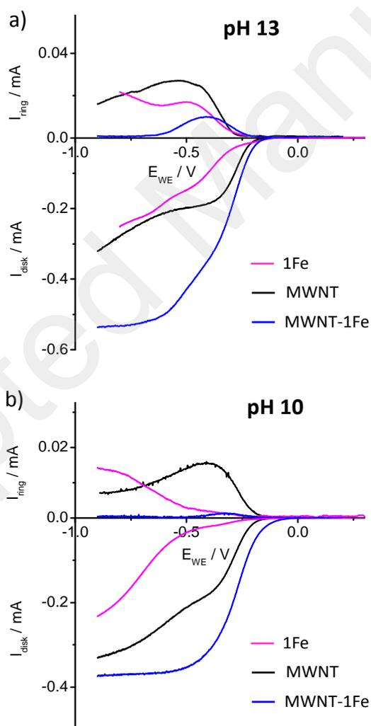
**Figure 5.** RRDE measurements of oxygen reduction (negative current) and hydrogen peroxide oxidation (positive current) for **MWNT** (black), **1Fe** (pink) and **MWNT-1Fe** (blue) at (a) pH 13 and (b) pH 10 in  $\text{O}_2$ -saturated solutions. The ring electrode was polarized at 0.260 V vs Ag/AgCl. Rotation rate: 400 rpm; scan rate: 5  $\text{mV s}^{-1}$ .
