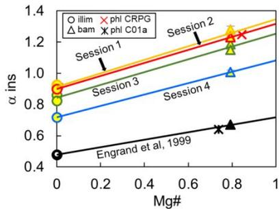
**Figure 5.** Instrumental fractionation factor on FIB sections of Illimaussaq amphibole (illim), Bamble amphibole (bam), and CRPG phlogopite (phl CRPG) during different sessions (represented by different colors). The results acquired by Engrand et al.<sup>34</sup> (shown in black) with an O<sup>-</sup> source, on both amphiboles and phlogopite C01a (phl C01a) are plotted for comparison.
