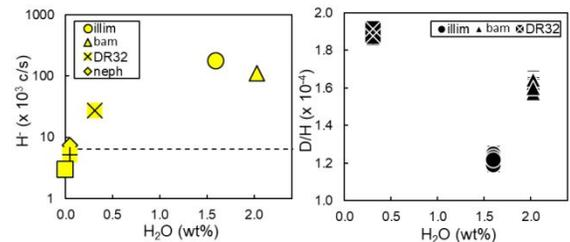
**Figure 7.** a) Hydrogen intensity of minerals prepared as FIB sections as a function of water content. The dashed line represents the hydrogen intensity for which the D count rate is only 1 c/s assuming a D/H ratio equal to the terrestrial reference. b) D/H ratio of minerals prepared as polished section and FIB sections as a function of water content. illim: illimaussaq, bam: bamble, DR32: DR32 glass, neph: nepheline, sod: sodalite, px: 71-98 pyroxene.
