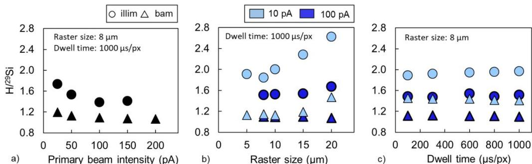
**Figure 2.** Evolution of  $H/^{29}Si$  ratio of bamble (bam) and illimaussaq (illim) amphiboles with a) primary beam intensity, b) raster size and c) dwell time.
