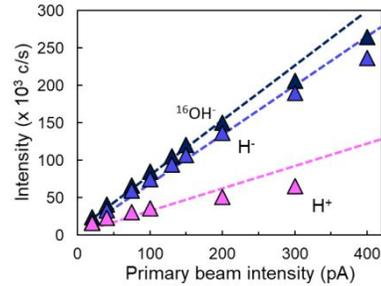
**Figure 1.** Evolution of the intensity of secondary ions with primary beam intensity on Bamble amphibole polished section mounted in epoxy.  $Cs^+$  primary beam is used to collect  $^{16}OH^-$  and  $H^-$  ions whereas duo source is used to collect  $H^+$  ions. All values are collected in the tuning of the CAMECA software. Dashed lines correspond to the linear relationship between secondary ion intensity and primary beam intensity below 100 pA.
