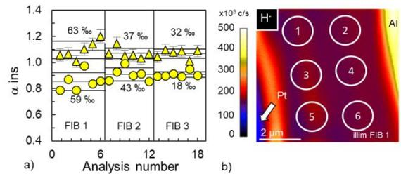
**Figure 6.** a) Instrumental fractionation factor of Illimaussaq (circles) and Bamble (triangles) amphiboles for six regions of interest (ROIs) in three distinct FIB sections. The standard deviation associated to a FIB section is noted next to the points. b) The hydrogen intensity image of the FIB section 1 of Illimaussaq amphibole is presented with the circular ROIs having a  $1.5 \mu m$  diameter.
