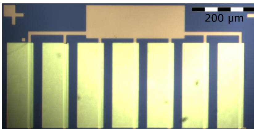
Figure S7. Optical microscope image of a typical final sample used for electrical measurements. The orange part is the grafted bottom electrodes, the yellow parts are top electrodes.
